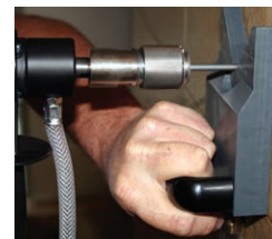
3-speed EBM 352/3 P (motor only, for use with compatible stands) EBM 352/3 PSA (anchor stand) EBM 352/3 PSV (anchor vacuum stand) Drill holes up to 14"***
