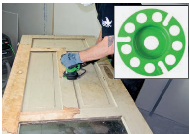
Carbide milling disc for wood surfaces (P/N 37124)
