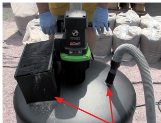
Pouring inlet tube and integrated dust extraction port reduce airborne dust while adding and mixing materials
