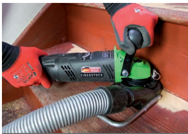
Carbide milling disc for wood surfaces (P/N 37124)
